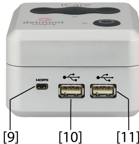
Figure 3 : control unit, back panel
